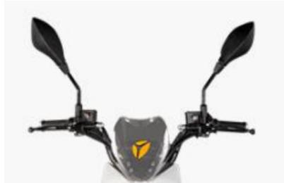
1. Mirrors can be easily fixed to the handle bars between the grips and the brake handle.
